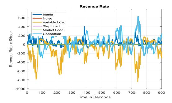
Figure 11: Rate of Revenue Accumulation in Toy System
