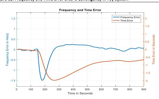
Figure 12: Frequency and Time Error after a Contingency in Toy System
