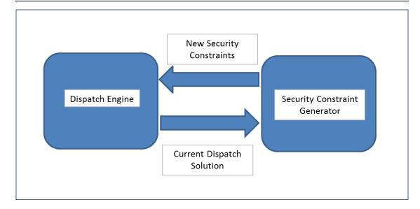
Figure 17: Dynamic Generation of Security Constraints
